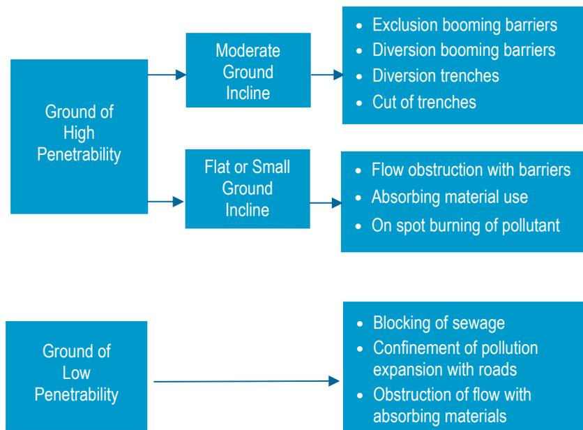
The efficiency of the above methods is impeded by the accessibility to the site, the required time for application, the rough and rocky terrain, the environmental consequences of excavations and the presence of natural water flow.
